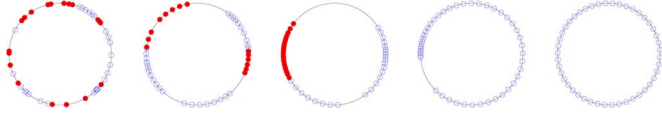
Fig. 1. The agree-and-pursue control and communication law in Section II-C with N = 45 , r = 2\pi/40 , and k_{\text{prop}} = 7/16 . Disks and circles correspond to agents moving counterclockwise and clockwise, respectively. The initial positions and the initial directions of motion are randomly generated. The five pictures depict the network state at times 0, 9, 20, 100, and 800.
