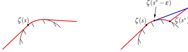
Fig. 14 At left, an example of a non-simple (time-optimal) path around an obstacle. At right, we provide a counterexample showing that a tangentially departing path is optimal.
