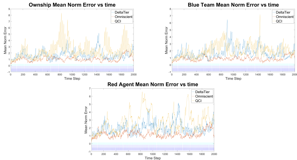
Fig. 7: Average ownship, blue team and red agent estimate norm error for the Omniscient, Delta-Tiering and QCI algorithms for each time step across 500 MC runs. The vertical lines at the bottom of the plots represent the acoustic modem activity. The tall cyan lines are the surface beacon's broadcast while the shorter magenta line and the shortest blue line are agent 1 and agent 2's triggering events respectively.
