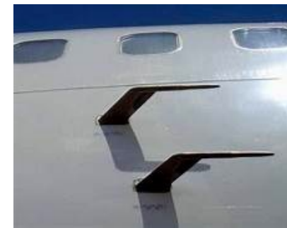
Pitot Tube on Aircraft
